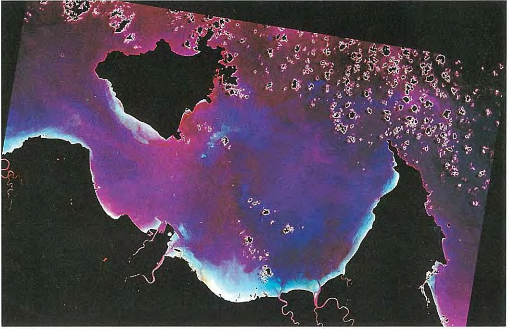
Figure 3 February 28 SPOT Satellite Image Clearly Shows the Sediment Plumes Associated with Dredging and the Off-shore Dump Ground
