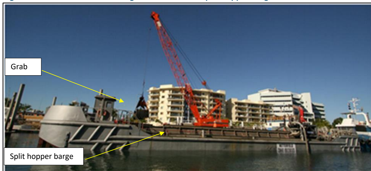
Figure 31: Mechanical Grab Dredge and Netterfield Split Hopper Barge
