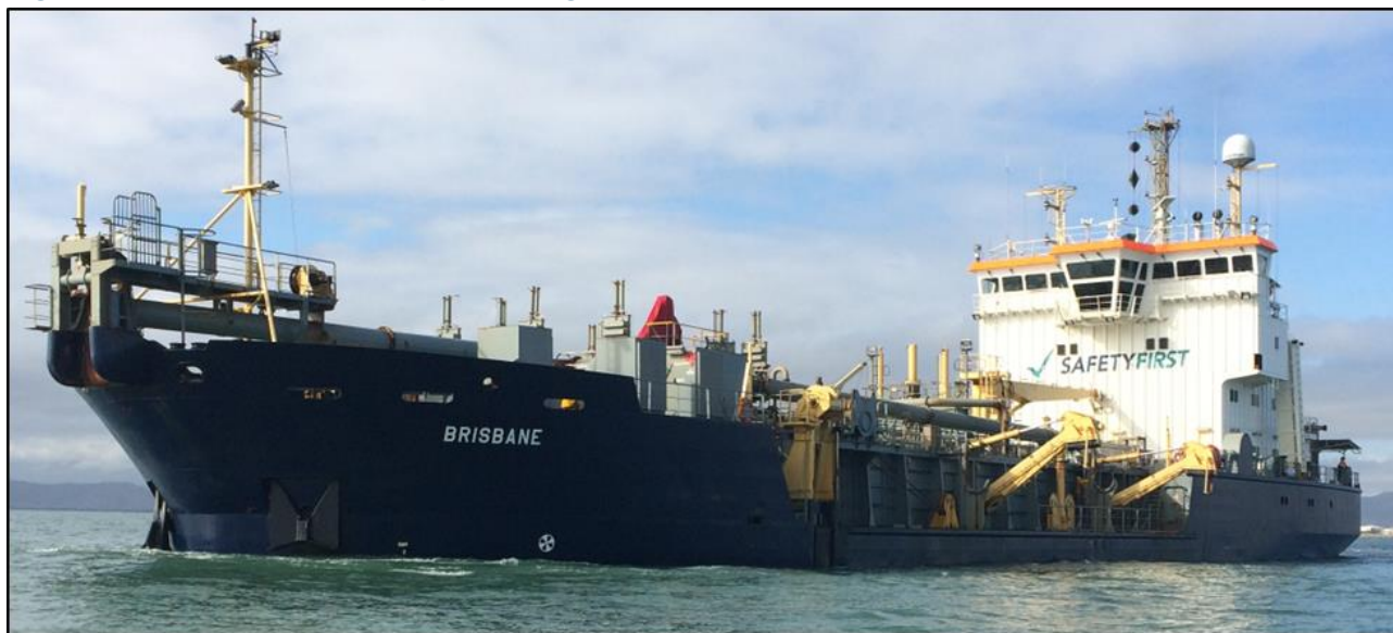
Figure 28: Trailer Suction Hopper Dredge Brisbane
