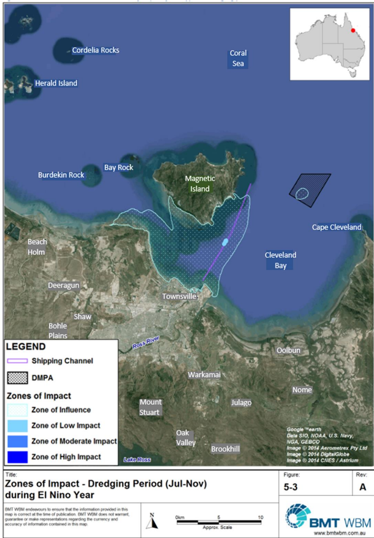
Figure 20: El Nino Year – Modelled Zones of Impact for a Typical Dredging Period
