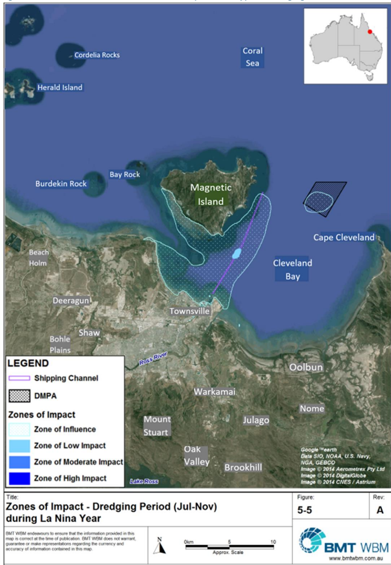
Figure 22: La Nina Year – Modelled Zones of Impact for a Typical Dredging Period
