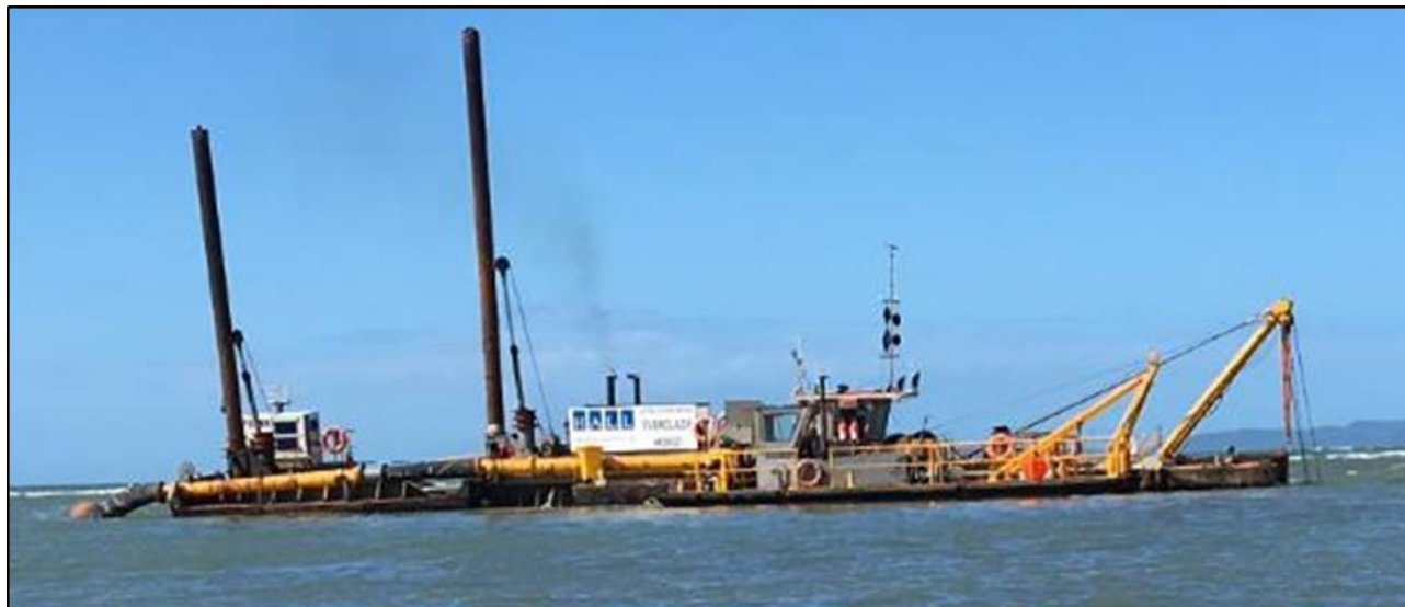
Figure 33: Cutter Suction Dredge Everglade
