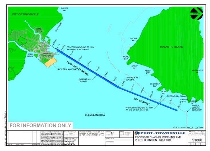
**Figure 2**. Site plan indicating the CCU project land reclamation area and proposed areas for widening of the existing channel (Map from Port Expansion Project EIS, Part A Project Description).
