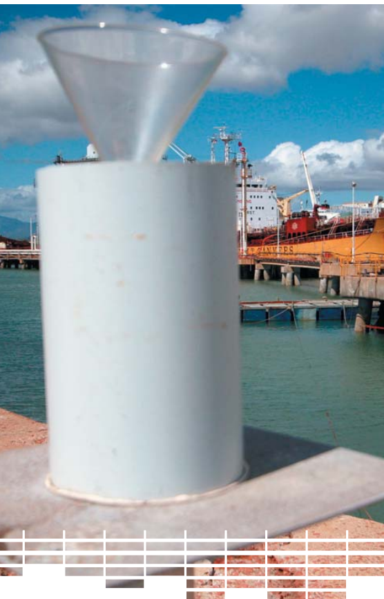
Dust deposition gauge at the Port of Townsville.
