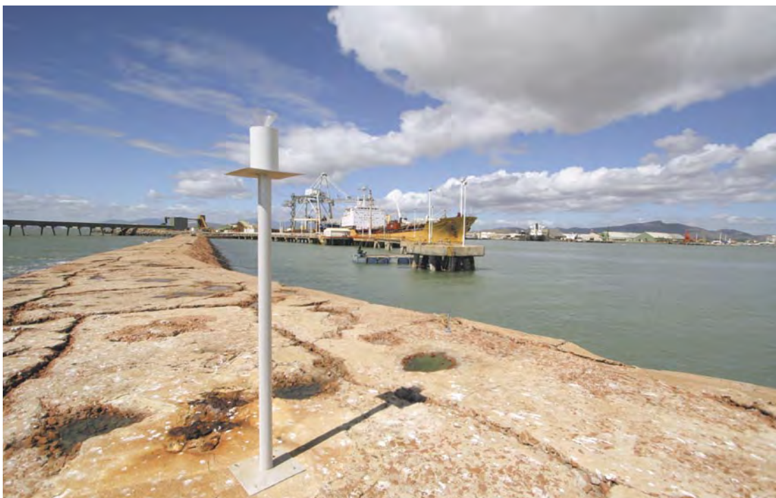
Ten dust deposition gauges are placed in strategic locations around the Port to supplement the dust monitoring program.
