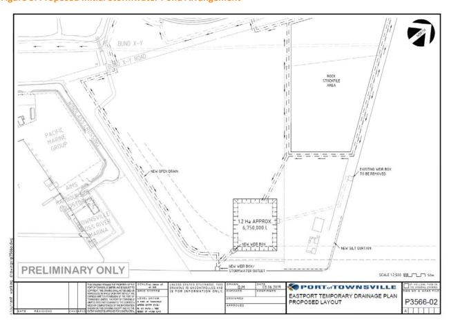
**Figure 5: Proposed Initial Stormwater Pond Arrangement**
