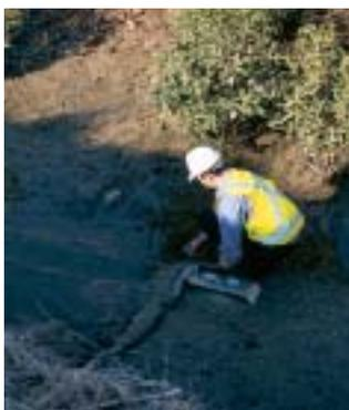
1 Craig Wilson checking stormwater discharge monitoring probes.
