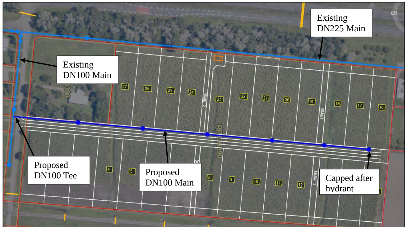
Figure 6: Proposed Water Main Layout
